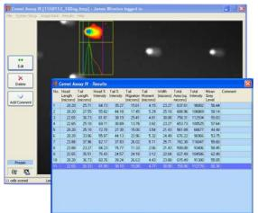
Measurements accumulated for each slide are viewable within a scrolling results window, which can be split from the main application and placed on a second screen in dual-monitor systems. The results window can also be hidden entirely for those wishing to score blind.
