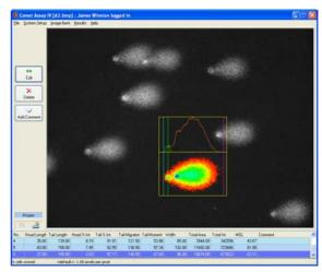
automatically compensates for slides with uneven backgrounds or varying levels of brightness, ensuring comparable results across a wide range of slides; even highly damaged 'hedgehog' comets can be accurately and consistently measured.
